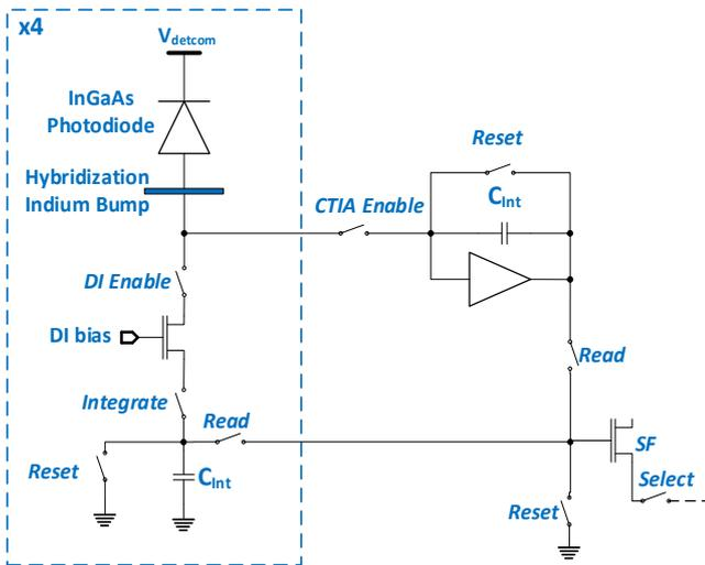
Fig. 1. Simplified imaging schematics
